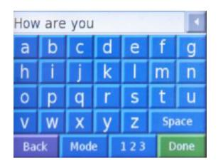
To create a message the driver is required to type a message using the touch screen keyboard. Once the message is complete the driver selects the Done button and the system confirms that the driver wants to indeed send the message. Some models provide canned messages the driver may select. These messages are set by the dispatcher.
